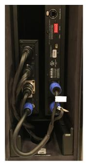
A Model A1 amplifier is powering the Model D speaker. The amplifier is mounted together with the crossover for the mid-high section in a chassis, which is fixed to the top of the box with two M4 screws.
