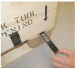
Pull out the Clip-Lok opening tool by using two fingers.
