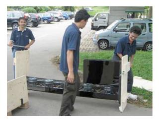
Place the steel levers into the lifting points like this.
